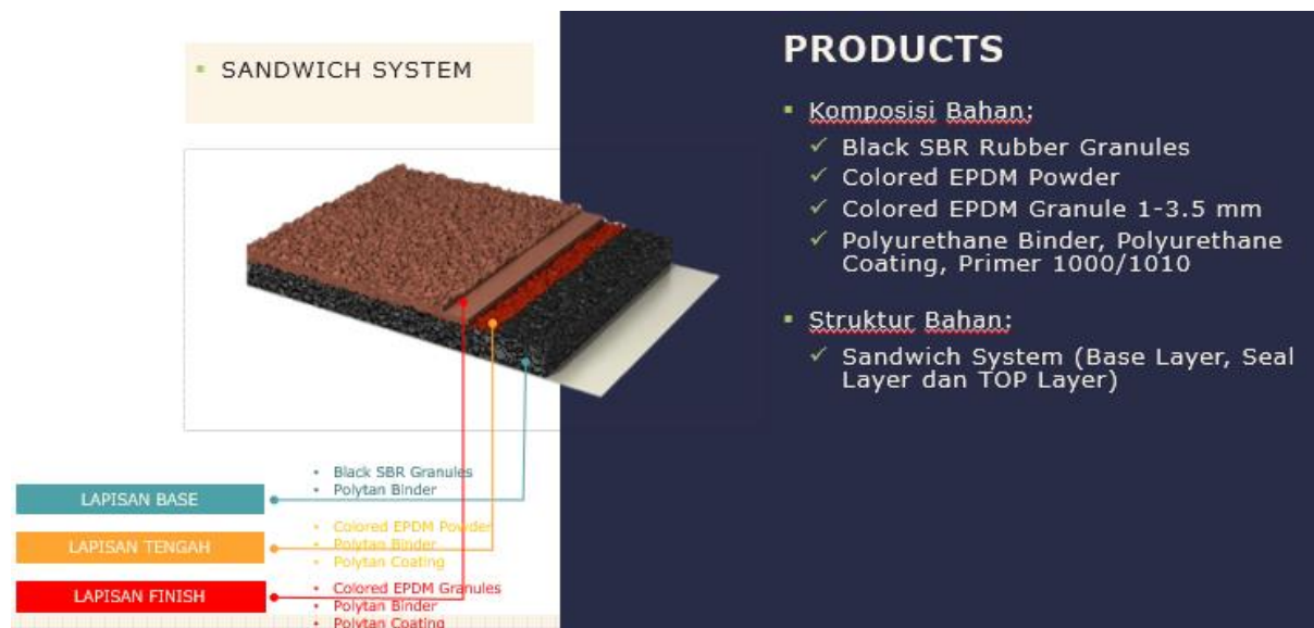
Gambar 2. Lapisan Sandwich System Track Atletik
