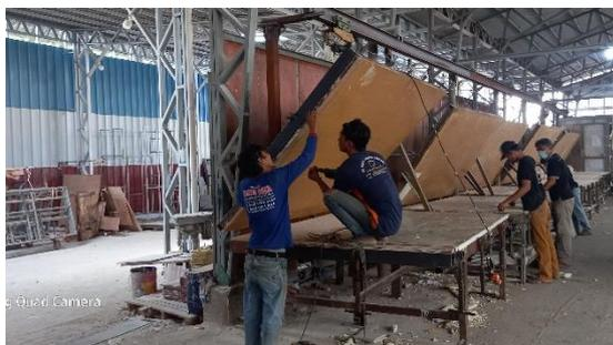
**Gambar 4.** Proses Pekerjaan Molding Dinding di Workshop
