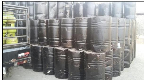
Gambar 3. Foto Asbuton Pracampur (aspabi.id)
