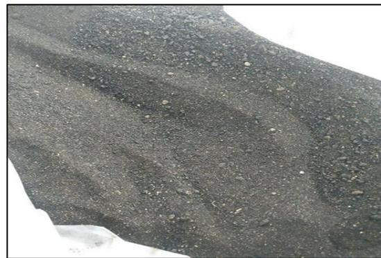
Gambar 1. Foto Asbuton B 5/20 ([aspabi.id](http://aspabi.id))
