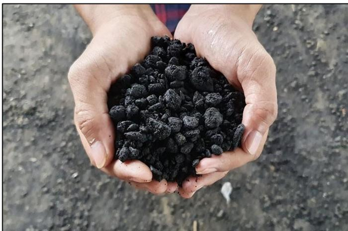
Gambar 6. Foto Cold Paving Hot Mix Asbuton/CPHMA (aspabi.id)
