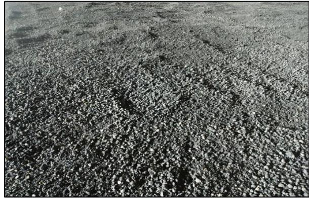
Gambar 2. Foto Asbuton B 50/30 (aspabi.id)
