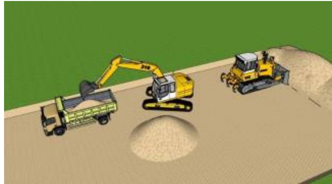
Gambar Pekerjaan galian tanah (Under Subgrade)
