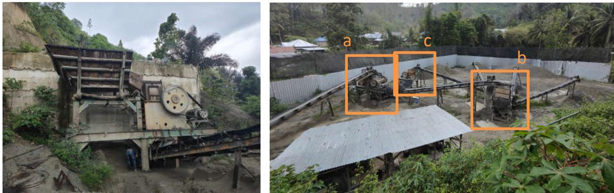
**Gambar 2. Primary, Secondary, Ayakan dan Tertiary Crusher**
