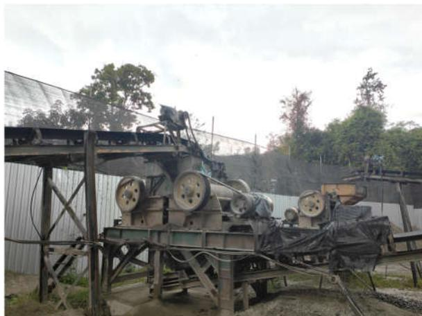
**Gambar 5. Secondary Crusher**
